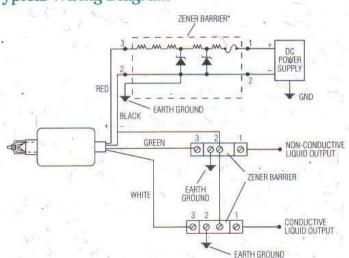
Source voltage not greater than 250 VAC. Zener barriers must be installed in accordance with barrier manufacturer's instructions.
