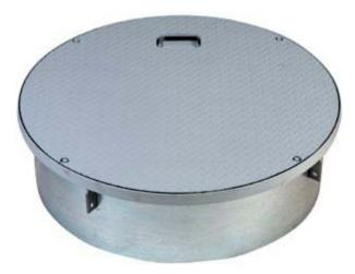
POMECO/OPW 110/120 Series Round Manholes are designed for use in a wide range of service station driveway, industrial, and commercial applications. The 110s and 120s are used to provide access to all types of underground equipment, including vapor recovery connections, UST monitoring equipment and submersible pumps. The 120 Series includes Roto-Lock fasteners on 24" and larger manholes.
