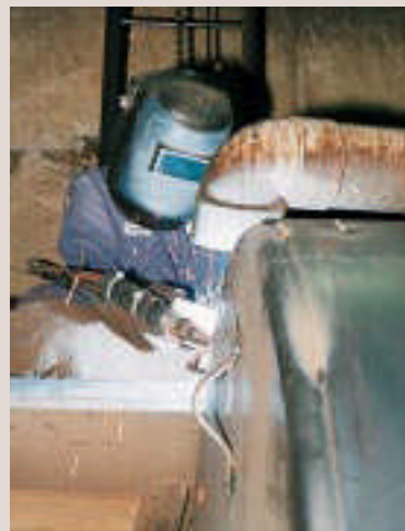
Welding All tanks are sealed with a continuous exterior full-fillet lap weld. Interior welding is available with interior coatings.
